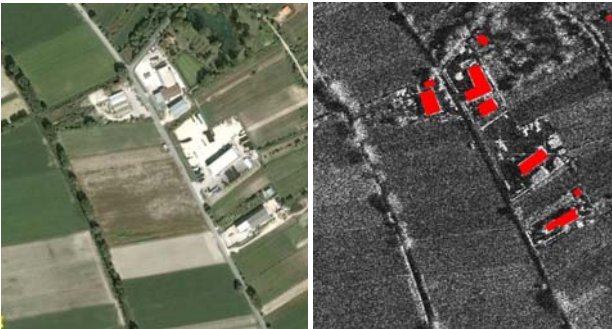
Fig. 2 Ground truth from Google Earth (left) and corresponding ROI overlapped to COSMO-Skymed image (right)
