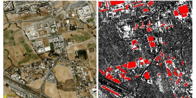
Fig. 4 Ground truth image from Google Earth (left) and corresponding ROI overlapped to TerraSAR-X image (right)
